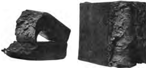
FIG. 17.—Fracture of Low Moor Iron, showing "fibre."
